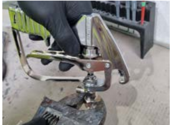
4. Tighten with wrench until tip is straight
