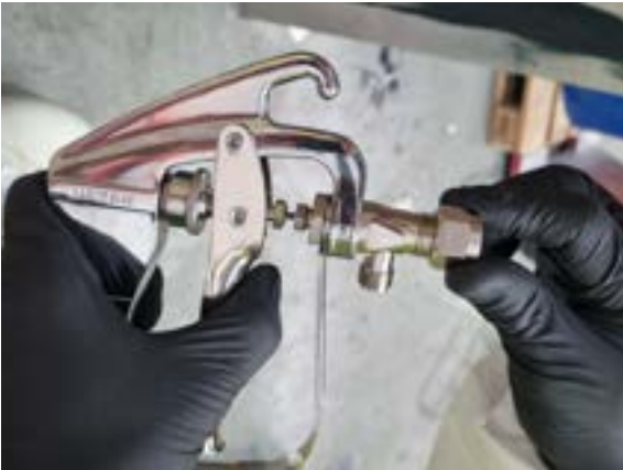
3. Lay tip retainer on top and screw on
