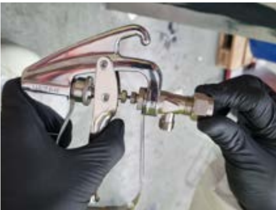
3. Lay tip retainer on top and screw on
