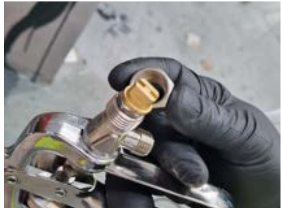
2. Lay spray tip on top
