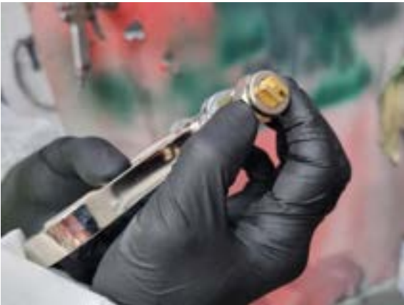
1. Unscrew tip retainer
